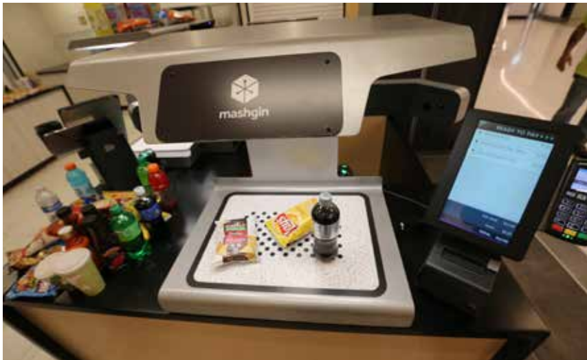
Able to recognize food items by their size, shape and color, the Mashgin self-checkout units speed up the check out process.
